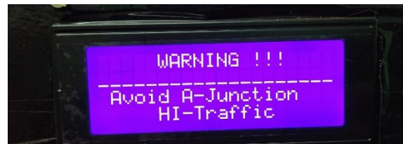
Figure 4.9: When Fire-service button is pressed
